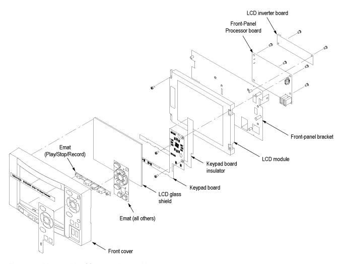
Figure 3-8: Disassembly of front-panel assembly
