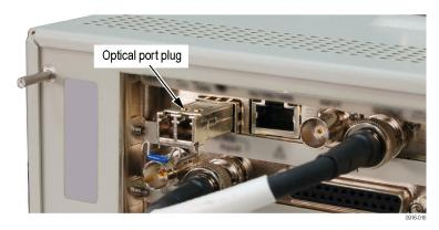
Figure 3-11: Removing the SFP module.
