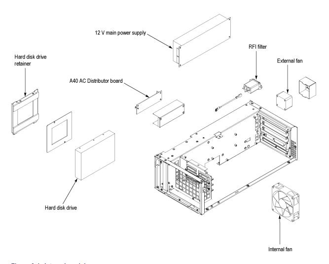
Figure 3-4: Internal modules
