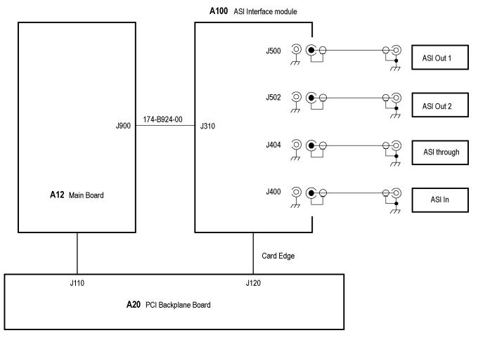
Figure 4-3: A100 ASI Interface module connections
