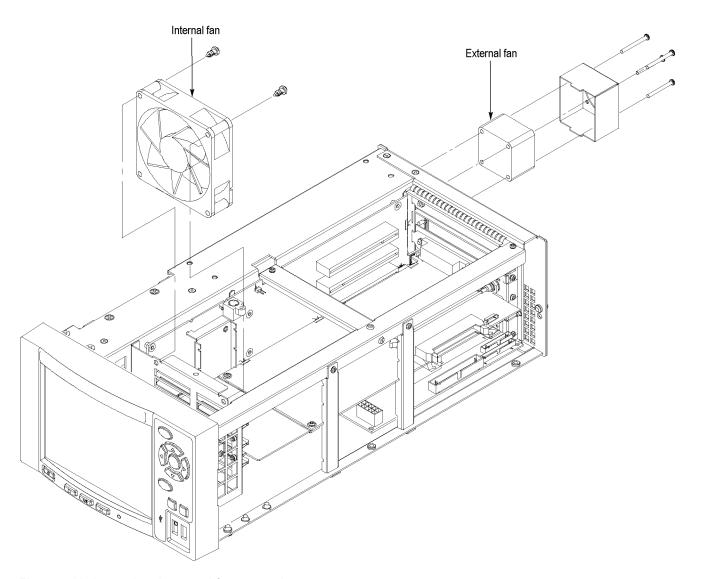
Figure 3-14: Internal and external fan removal
