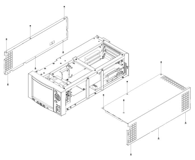
Figure 3-6: Right-side and left-side covers removal
