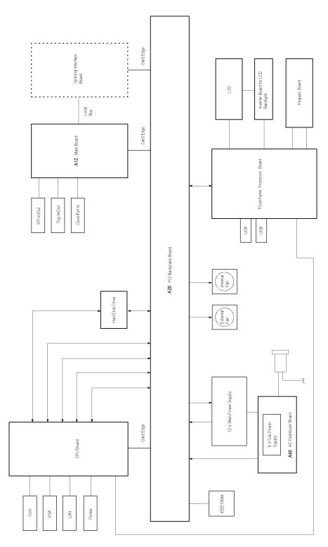
Figure 4-1: MTX100B block diagram
