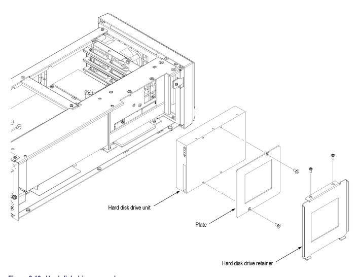
Figure 3-13: Hard disk drive removal
