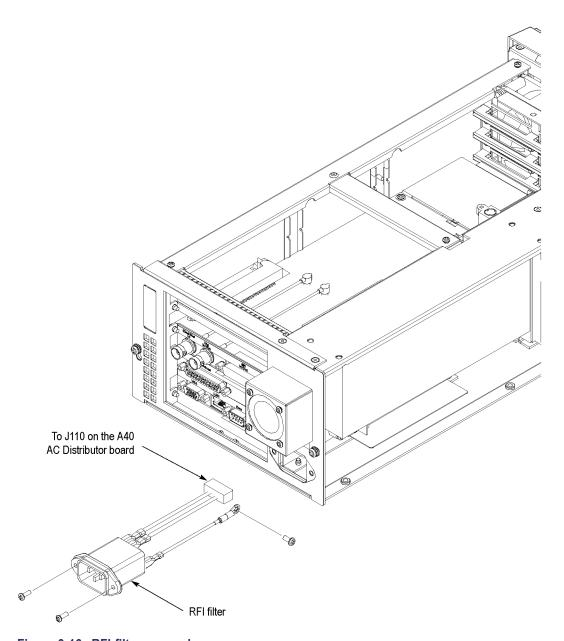
Figure 3-16: RFI filter removal
