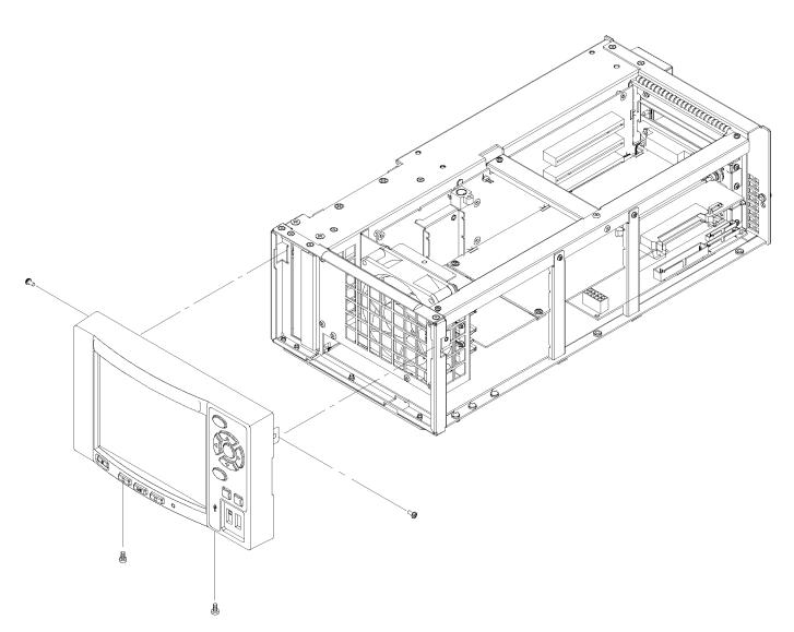
Figure 3-7: Front-panel unit removal
