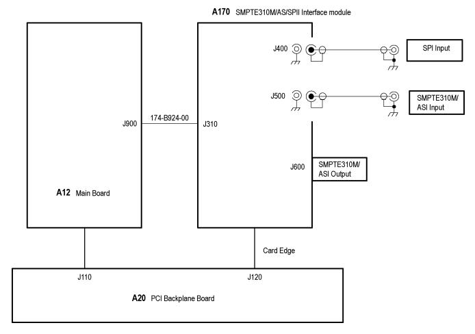
Figure 4-6: A170 SMPTE310M/ASI/SPI Interface module connections
