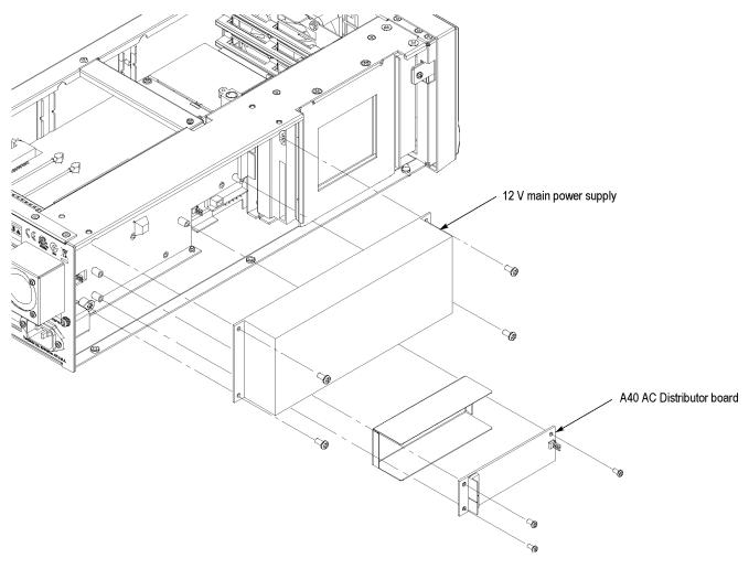
Figure 3-15: 12 V main power supply and A40 AC Distributor board removal
