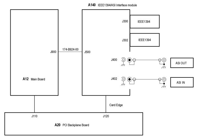
Figure 4-5: A140 IEEE1394/ASI Interface module connections
