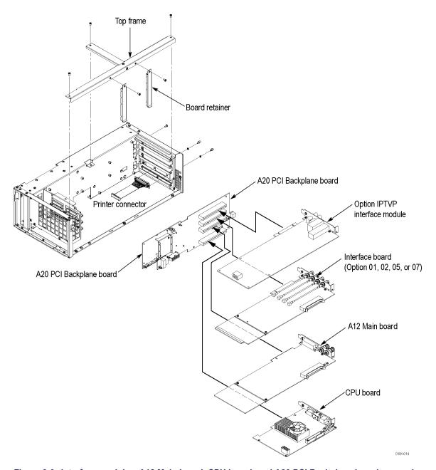
Figure 3-9: Interface modules, A12 Main board, CPU board, and A20 PCI Backplane board removal
