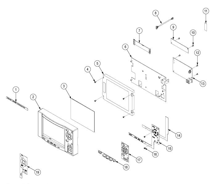
Figure 5-4: Front-panel unit
