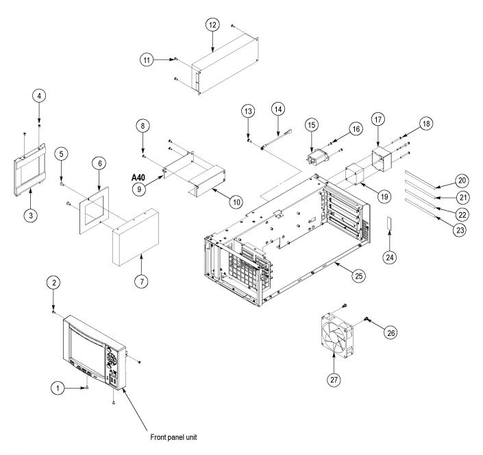
Figure 5-2: Internal modules
